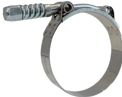
T-bolt clamp with spring can provide constant tension performance to compensate for the expansion and contraction when temperatures fluctuate. Provides high strength and a 360° seal. Designed for use in high vibration and large diameter applications common in heavy trucks, industrial machinery, off road equipment, agricultural irrigation and machinery, for air intake and coolant adapter.
